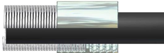
3. Insert the second piece of flexible armour into the other side of the Armour Joint until it also reaches the internal stop.
