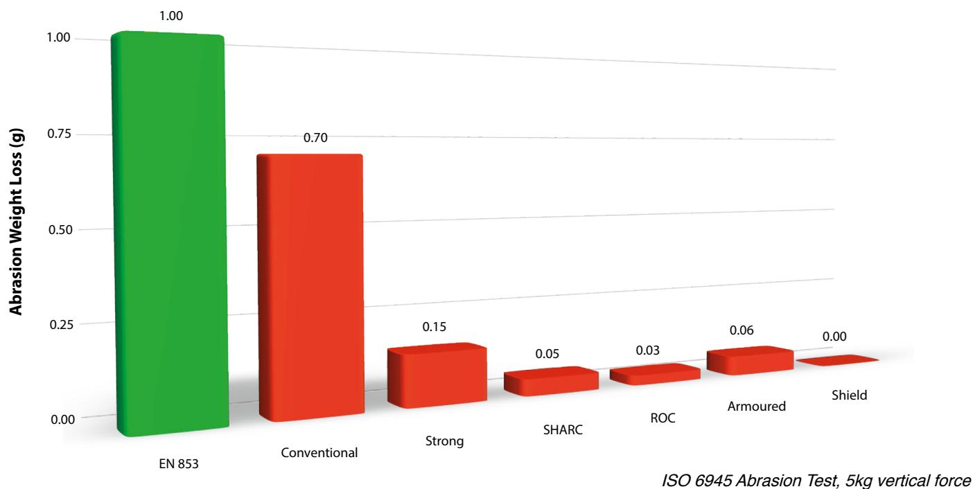
In addition to their outstanding performance against abrasion, these covers also boast a high level of resistance to cracking due to ozone exposure. The general rule of thumb is that abrasion resistance and ozone resistance for a cover compound are inversely proportional. So high abrasion resistance leads to poor ozone resistance, and vice versa.
