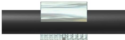
2. Insert the first piece of flexible armour into the Armour Joint until it reaches the internal stop.
