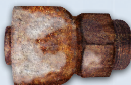
Competitor B after 1,000 hours ASTM B117 (ISO 9227) salt spray test
