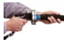
clamp tool for FrigoClic fittings
